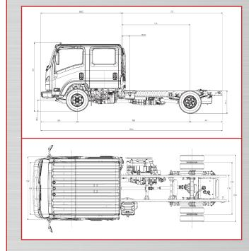
Wheelbase (in.) Cab to Cab to End Back of Overall Overall Axle Overall Body Axle (in.) of Frame (in.) Cab (in.) Length (in.) Length (in.) Width (in.) Width (in.) Height (in.) 150.0 131.6 241.5 81.3 88.5 5.3 12 65.6 92.4 114.5 157.6 5.3 267.5 81.3 65.6 92.4 176.0 16
